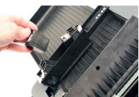
3. Pull the cartridges out of the cartridge holders using the cartridge tab.
